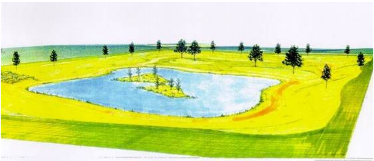
Figure DB-2. Water Quality Detention Pond Incorporating Wet Pond and Natural Contours
